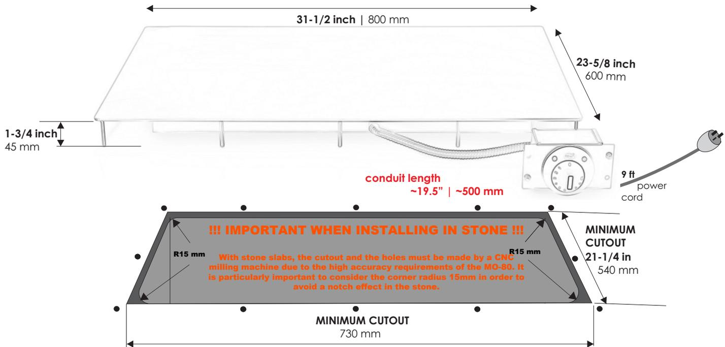
▶▶ The Control Box **MUST** be firmly fastened to a **NON-MOVING** surface. Conduit + power cord to be secured.
